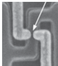
Silicon NanoMOSFET with two gates separated by 16 nm fabricated using the LETI facility
