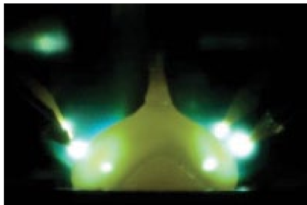
Crystal growth of UCoGe in a new tetra-arc furnace, a recently discovered ferromagnetic superconductor, for high pressure and high field investigations
