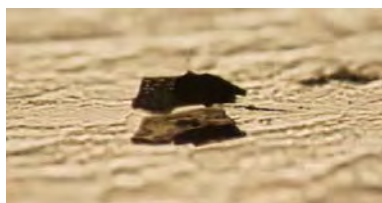
Fig. 1: a 5 \mu\text{m} thick magnet in levitation above graphite (G2ELab-NEEL)
