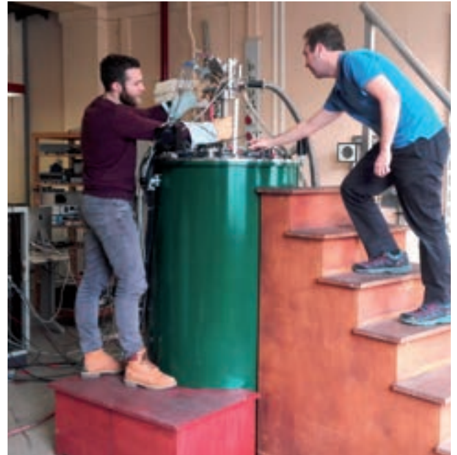
Fig. 2: Heat capacity measurements on superconductors using the 20 T magnet.
