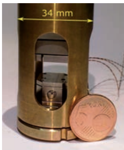
Fig.1: the compact scanning probe microscope.
