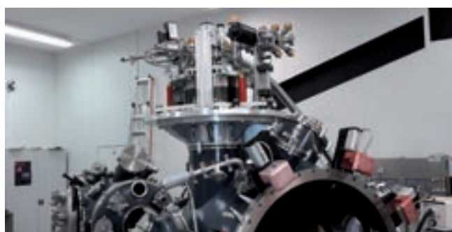
Fig. 1: A view of the cryostat installed on the laser PALS.
