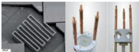
Fig. 1: Capacitive sensors: left: zoom of a silicon spring of the MEMS sensor. right: «macroscopic» sample holder, fabricated with a 3D printer.
