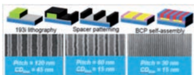
Fig. 1: ICTs: DiSABloC's BCP chemo-epitaxy flow based on spacer patterning leading to 30 nm pitch line patterns
