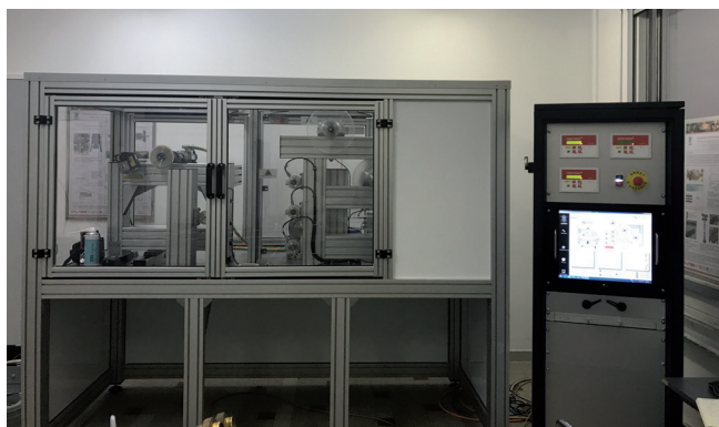
Fig 1: The HTS winding machine during operation
