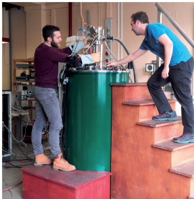
Fig. 2: Heat capacity measurements on superconductors using the 20 T magnet.
