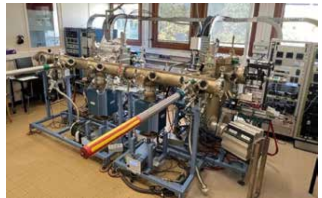
Figure 1: Photograph of the 2D cluster with Se and Te MBE reactors connected by a UHV transfer tube.
