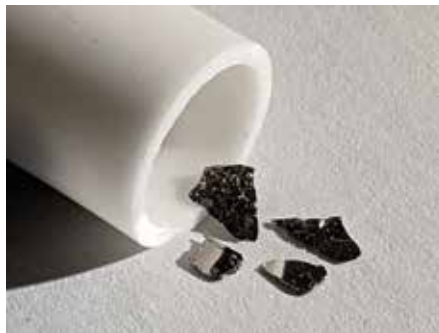
Fig.1: Crystals of LaNiGa_2 next to the alumina crucible in which they were synthesized.
