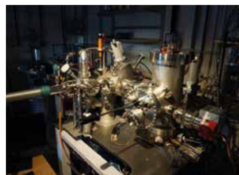
Fig. 1: The present mK STM setup. Within this project, the dilution refrigerator (right part of the setup) will be made fully UHV compatible.
