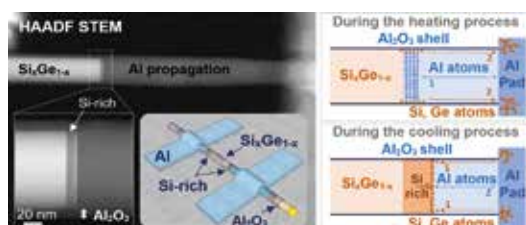
Fig 1: Scanning TEM images of a propagated NW passivated with 20 nm of \text{Al}_2\text{O}_3 and an inserted schematic showing the formation of Al/Si-rich/ \text{Si}_x\text{Ge}_{1-x} heterostructures [2].
